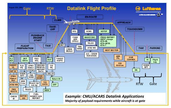
Figure 9: ACARS Datalink Applications
