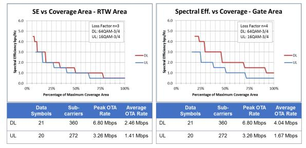
Figure 4: Spectral Efficiency and Over-the-Air Data Rate
