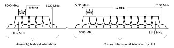
Figure 1: AeroMACS Channels Are Defined across 5000-5150 MHz of which 5091-5150 MHz Was Internationally Allocated by ITU in 2007
