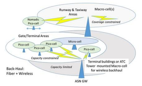
Figure 6: A large airport has varied BS requirements for coverage and capacity
