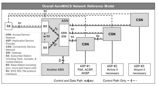
Figure 2: Overall Network Reference Model
