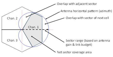
Figure 7: Sector or Channel Coverage for 15 dBi BS Sector Antenna
