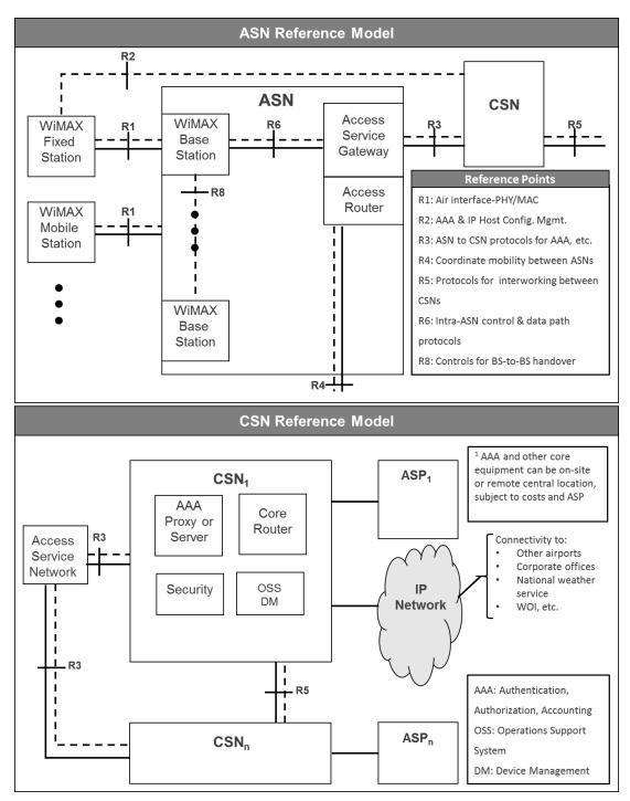
Figure 3: Detailed AeroMACS ASN and CSN Reference Model
